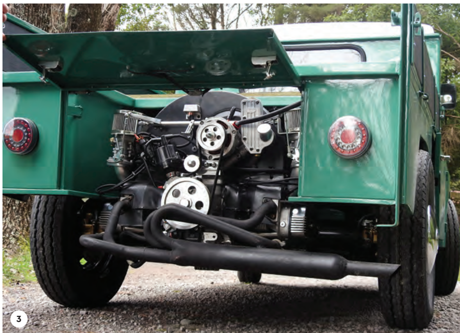
1. The Mactra showing off its simple lines (Photo Patrick Harlow); 2. Rear view of the Mactra (Photo Patrick Harlow); 3. Exposing the Mactra's air-cooled VW engine (Photo Patrick Harlow); 4. The Mactra's no-nonsense cabin (Photo Patrick Harlow); 5. Like the donor VW, the Mactra's fuel tank was located up front (Photo Patrick Harlow).
