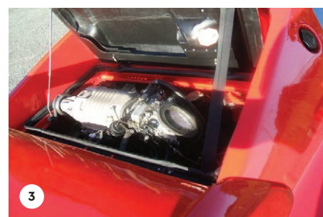
1. Spoilers and side skirts were not part of Ross Baker's original design (Photo Patrick Harlow); 2. Dramatic rear three-quarter view of the 2+2 Heron (Photo Patrick Harlow); 3. Cramped engine bay filled with a supercharged 3.0-litre Mitsubishi V6 (Photo Patrick Harlow); 4. Telstar instrument cluster finishes the Heron's supercar look (Photo Patrick Harlow).
