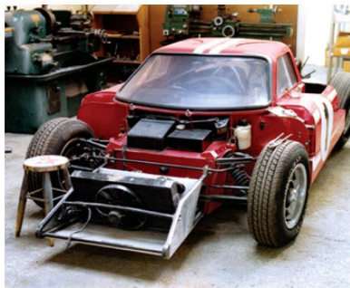
Below and right: Pictures from the original 1967 build with Corvette V8, suspension detail, and the locally created transaxle
