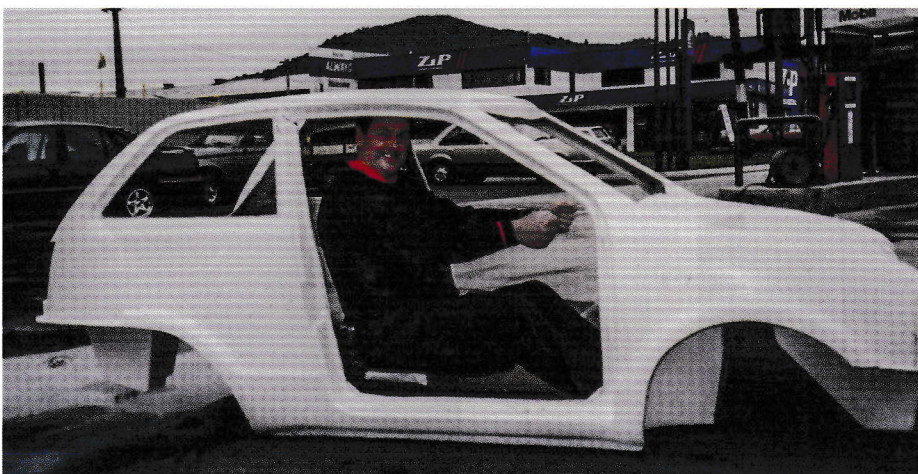
Left: Plug for the fibreglass moulds takes shape Below: Ross tries out body-number-one for size
