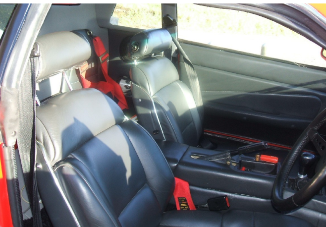
Grey leather seats are custom made for comfort. A full racing harness has also been fitted to this car.
