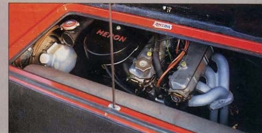
Don Hague's Immaculate MJ1 is one of the last of the original run of 24 cars. Mid-mounted two litre Fiat twin-cam provides 85 kW, more than enough urge for 750 kg coupe
