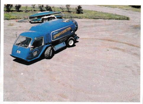
Spraymaster number one: The traditional problem of four-wheel drive vehicles requiring large turning circles has been eliminated with four-wheel steering. The 7.3 (24ft) turning circle from the outside of the tracks enables the sprayer to turn from one row into the next in one movement. The rear wheels track identically behind the front ones so there is no corner-
