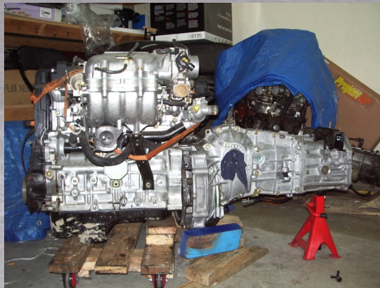
Right and Bottom: The Heron as it looked outside my garage recently. Below: The 2.2-litre Honda engine with the Subaru WRX transaxle.
